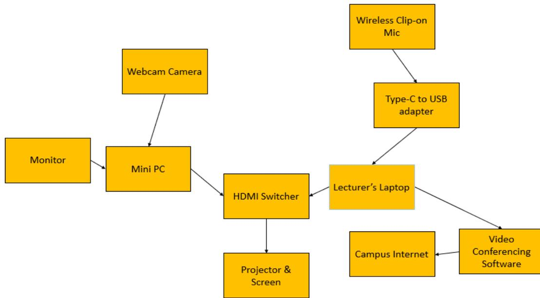
Figure 1. Hybrid Classroom System Diagram in Room A101
