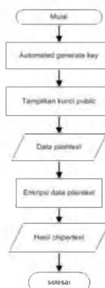
Gambar 3. Flowchart enkripsi data *plaintext*
