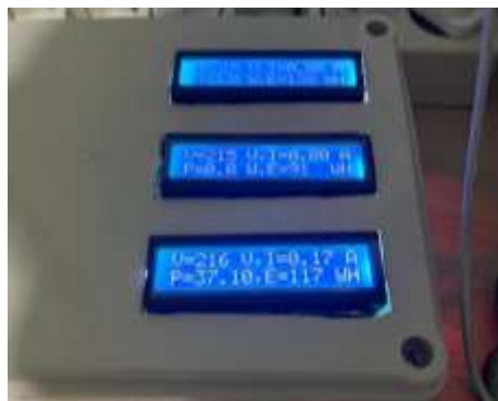
Figure 2. Testing Using Sensor PZEM-004T
