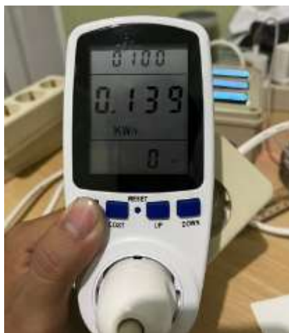
Figure 4. Testing Using a Digital Watt Meter
