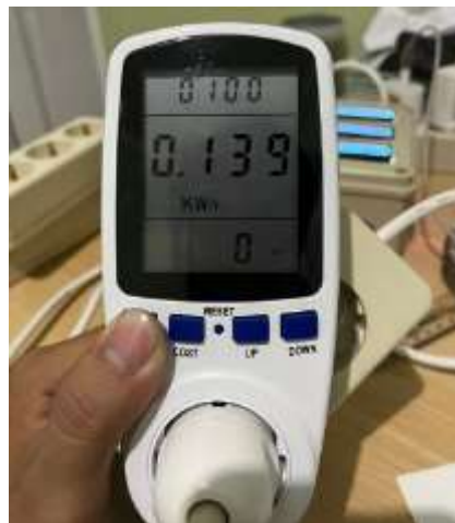
Figure 4. Testing Using a Digital Watt Meter
