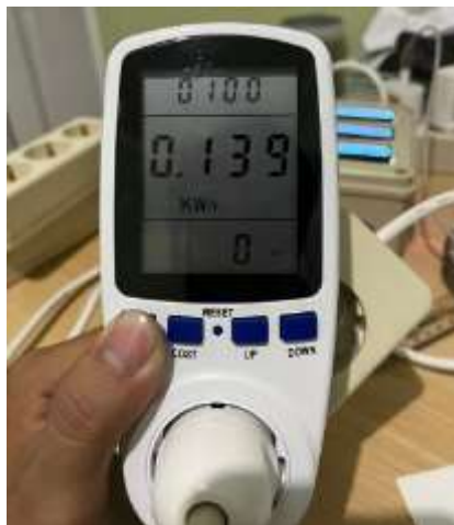
Figure 4. Testing Using a Digital Watt Meter
