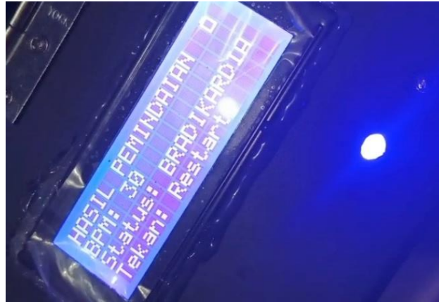
Figure 3. LCD display during ECG signal testing
