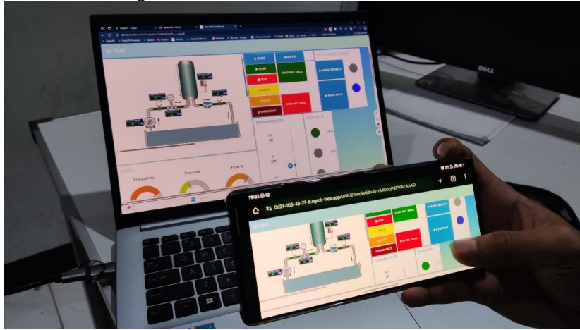
Figure 19. IoT Water Level Plant Hosting Testing
