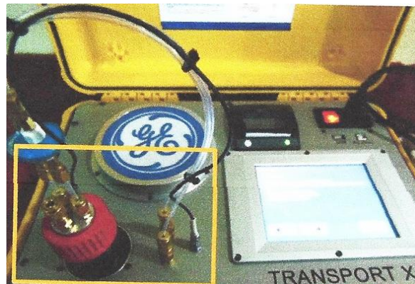
Figure 3. Dissolved Gas Analysis (DGA) measuring instrument
