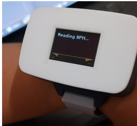
Figure 6. Wearable device prototype with sensor integration and OLED feedback
