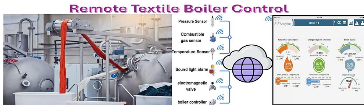
Figure 3. Remote textile boiler control system
