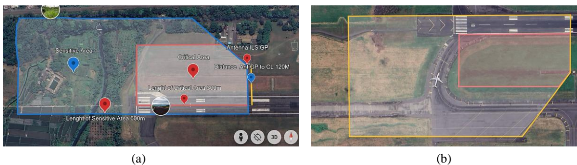
Figure 14. Observation of Siting Criteria for ILS GP: (a) Yogyakarta and (b) Surabaya
