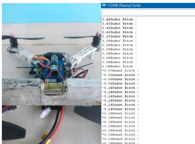
Figure 4. The testing of MPU6050 sensor against a measuring instrument
