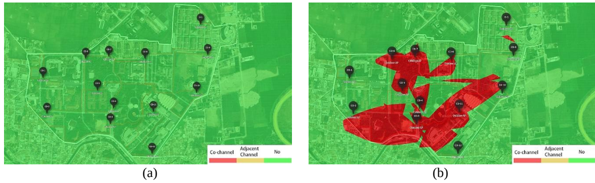
Figure 7. Heatmap of simulated interference in frequency band (a) 2.4 GHz and (b) 5 GHz
