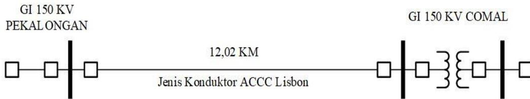
Gambar 1. *Single Line Diagram* SUTT 150 kV Pekalongan-Comal
