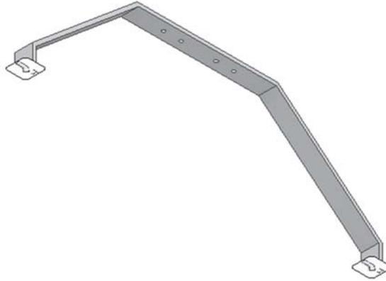
**Gambar 2.** Lokasi *fixed constraint* rangka main landing gear.
