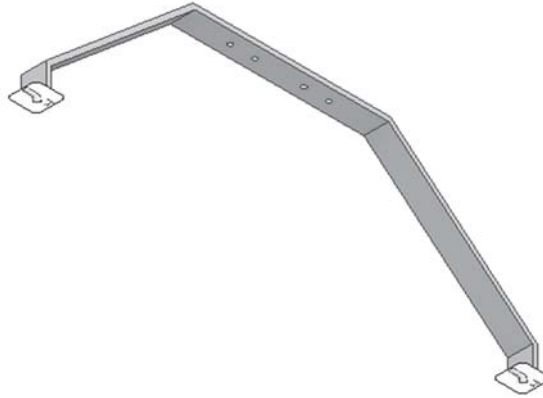
Gambar 2. Lokasi fixed constraint rangka main landing gear.
