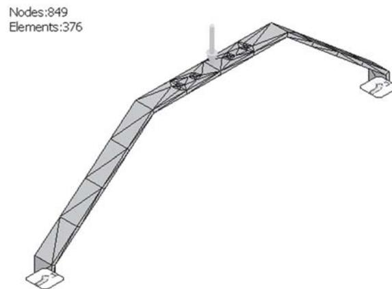
**Gambar 3.** Proses *meshing* rangka main landing gear.
