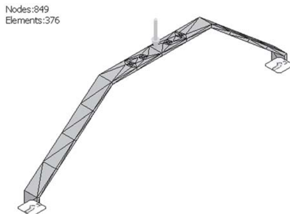
Gambar 3. Proses meshing rangka main landing gear.
