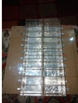
Gambar 1. Desain Aluminium Air Battery
