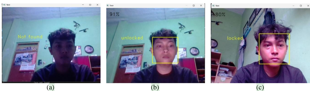
Gambar 9. Output Not Found (a), Unlocked (b), Locked (c)
